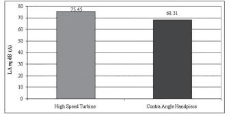
Figure 2: Mean noise levels of high-speed turbine and contra angle handpieces
