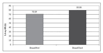
Figure 1: Average noise levels of used and brand new dental turbine compared
